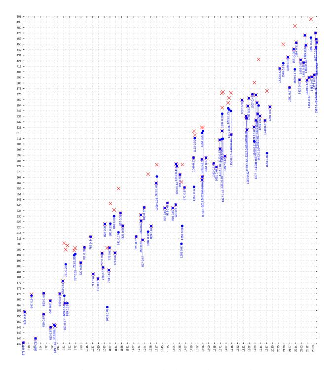
Figure 8: Estimated pre-quantum security level against known attacks, assuming sievingbased model of BKZ- $\beta$  cost, accounting for real cost of memory. Label: p, w/p. Horizontal axis:  $p \log_{256}((q+2)/3)$ . Log scale. Red: Ignoring hybrid attacks. Blue: Including hybrid attacks. See text for caveats regarding estimates.
